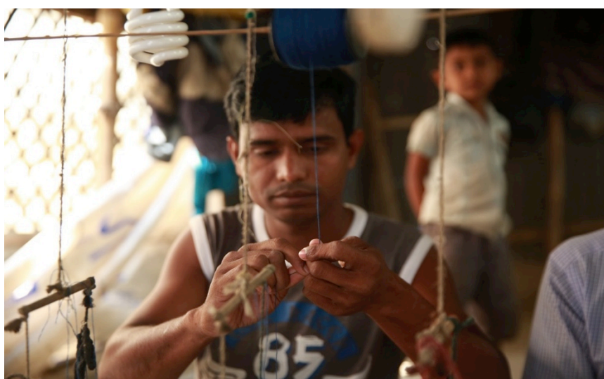
Figure 2: To create the Jamdani weave, Jabbar uses a bamboo splinter (as one would a needle) to combine weaving, embroidery and ornamentation.
